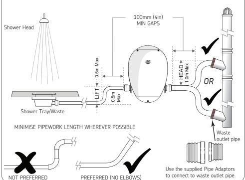
Important: Pipe connections must be easily accessed and pipework must be secured to prevent vibration and noise.
