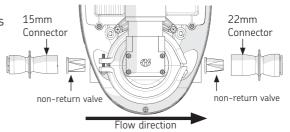
(8) Check that you have not overtightened and distorted the non-return valves before connecting the pipework. Refit the front cover.
