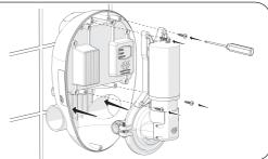
7 Fit the non-return valves as shown. Fit the pump connectors to the pump. Note 15mm connector for the inlet.
